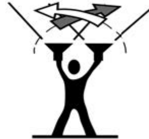
LZ UNSAFE (NIGHT)
