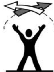
LZ UNSAFE (DAY)
